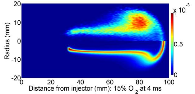
Figure 5: Comparison of OH mass-fraction contour between well-mixed (down) and PDF (up) models under 15%  $O_2$ ,  $14.8 \text{ kg/m}^3$  at 4 ms, PDF model with MC mixing model and  $C_\phi = 2.5$ .
