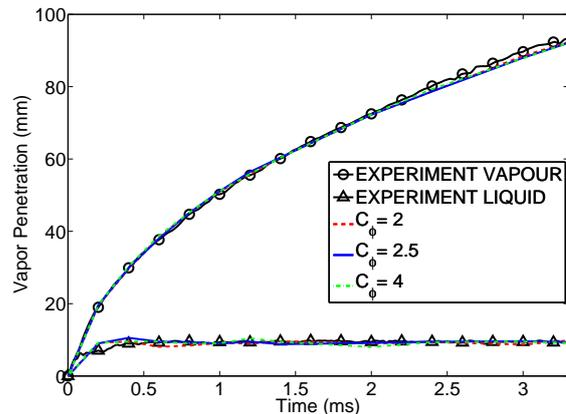
Figure 1: Vapour penetration and liquid length from experiments and computations with different mixing constants, MC mixing model.
