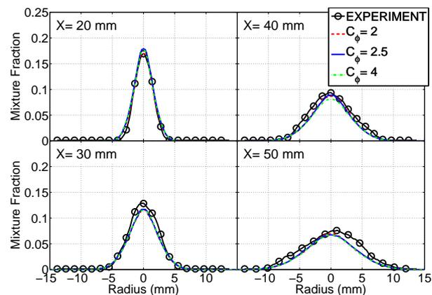
Figure 2: Radial profile of fuel mixture fraction from experiments and computations with different mixing constants, MC mixing model.
