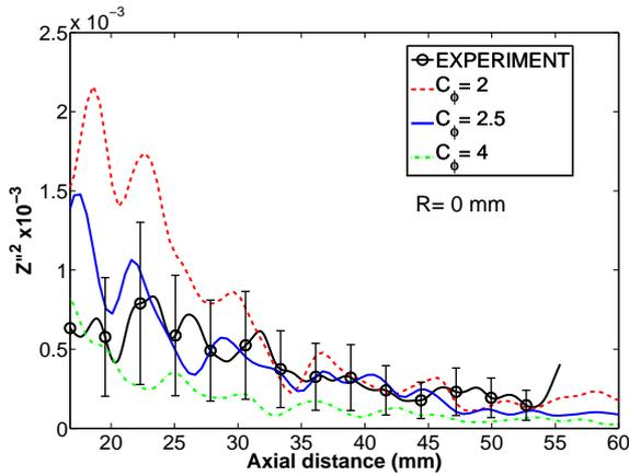
Figure 4: Axial profile ( $R = 0$  mm) of fuel mixture-fraction variance from experiments and computations with different mixing constants. The 95 % confidence interval is shown for the experimental data.
