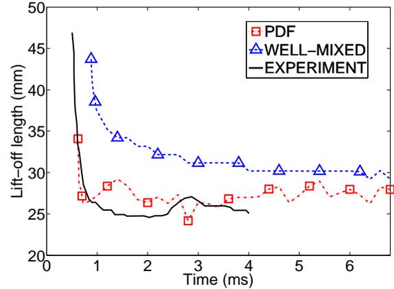
Figure 6: Comparison of temporal evolution of lift-off length between the well-mixed and PDF models under 15%  $O_2$ ,  $14.8 \text{ kg/m}^3$ , MC mixing model with  $C_\phi = 2.5$ .
