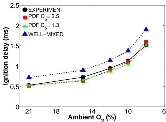
Figure 8: Comparison of ignition delay between well-mixed and PDF models under different ambient O<sub>2</sub> conditions at 14.8 kg/m<sup>3</sup>, PDF model with MC mixing model and different mixing constants.
