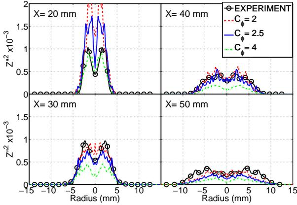
Figure 3: Radial profile of fuel mixture-fraction variance from experiments and computations with different mixing constants, MC mixing model.
