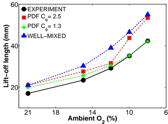
Figure 7: Comparison of lift-off length between the well-mixed and PDF models under different ambient O<sub>2</sub> conditions at 14.8 kg/m<sup>3</sup>, PDF model with MC mixing model and different mixing constants.
